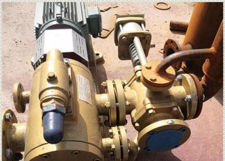
The 3QGB series heat-preservation high-viscosity three-screw pumps are mainly used to convey high-viscosity lubricating fluids. They are usually used as the delivery pumps of asphalt, heavy fuel oil, heavy gear oil and heavy diesel fuel. Inside the pumps, heat preservation chamber and channel are set us, gas or liquid could be used as heat carrier, and their maximum working temperature is equal to or lower than 350°C. High viscosity reduction, and the conveying viscosity is generally 3.0~760mm2.
