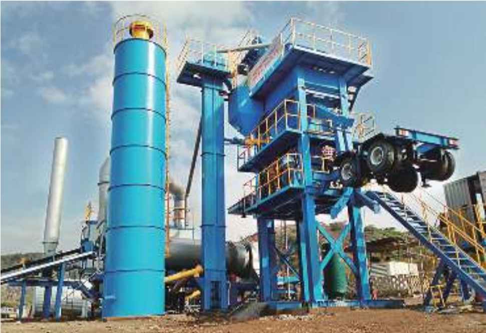
YLB700 Mobile Asphalt Mixing Plant in Ethiopia
